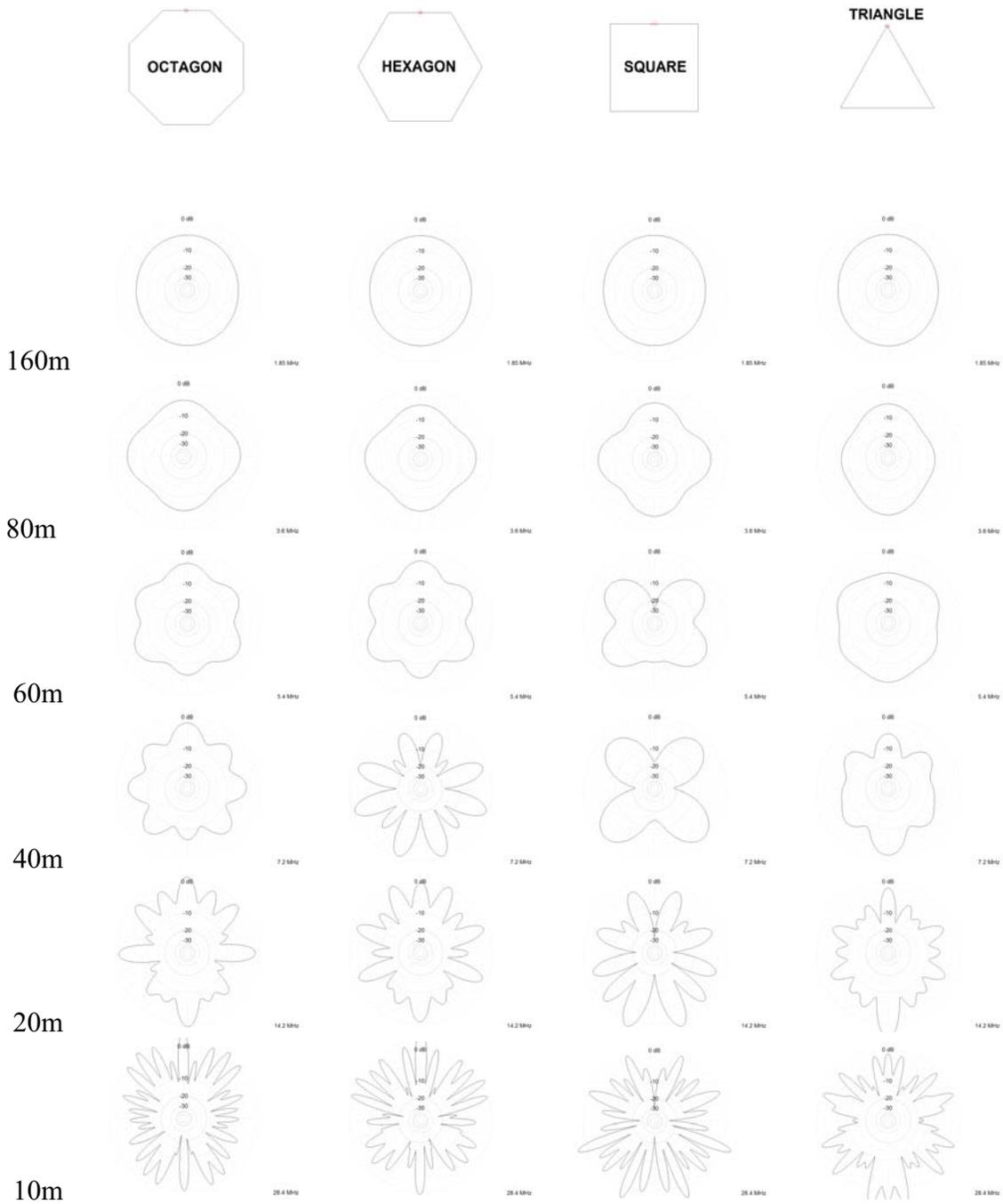
Figure 5. Horizontal Total Field Patterns for Long Wire Loops of One Wavelength Circumference on 160 meters (546-ft). All Antenna Models are at an Installed Height of 50-ft over Average Ground. Outer Ring is +10dBi for all Plots.
