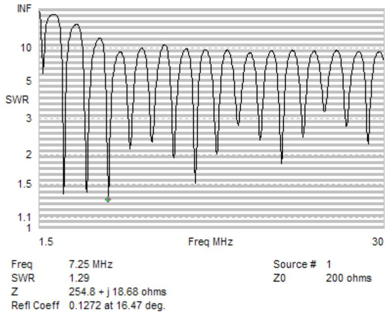
Figure 4. Swept SWR graph of a Long Wire Loop Showing Resonances on All Harmonics. The Loop is Fundamentally Resonant on 160 meters.
